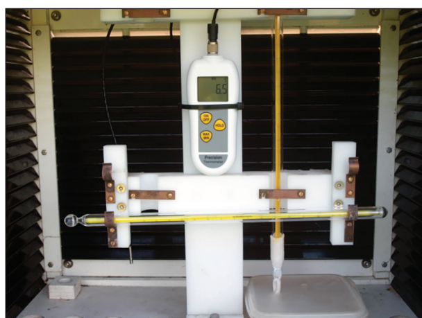
Thermometers inside Stevenson's Screen on the last day of 2017 Picture by Clive Cooper
