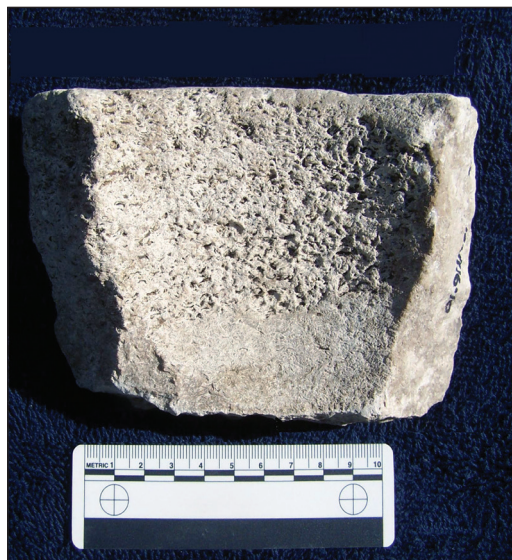
Plate G. Fragment of Bembridge Limestone mortar showing a lithological change towards the base. Context 160.
